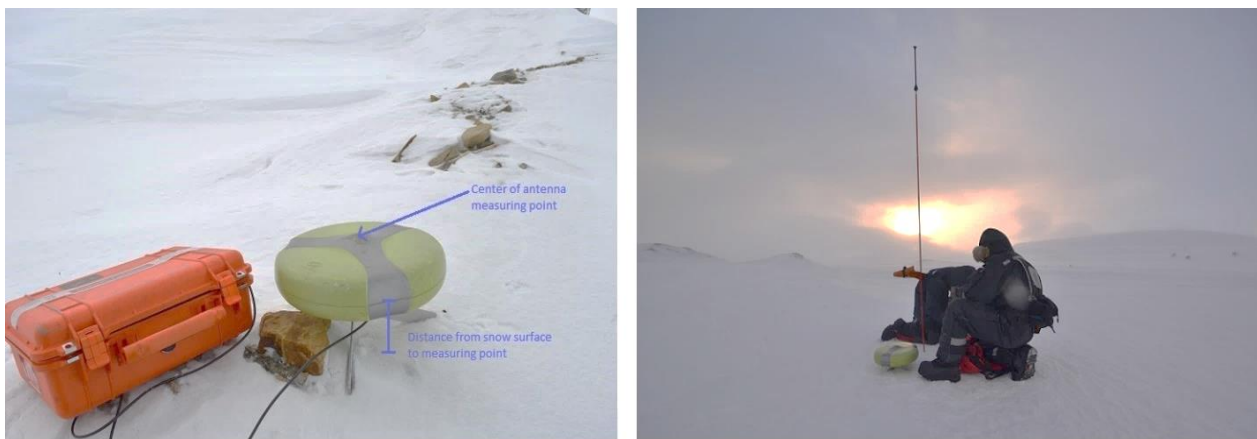
Figure 10: JAVAD RegAnt receiving GNSS satellite data showing the antenna measuring point axis and measured distance to the snow surface (left). Snow probing procedure over a GCP location in Sval1 area (right).
