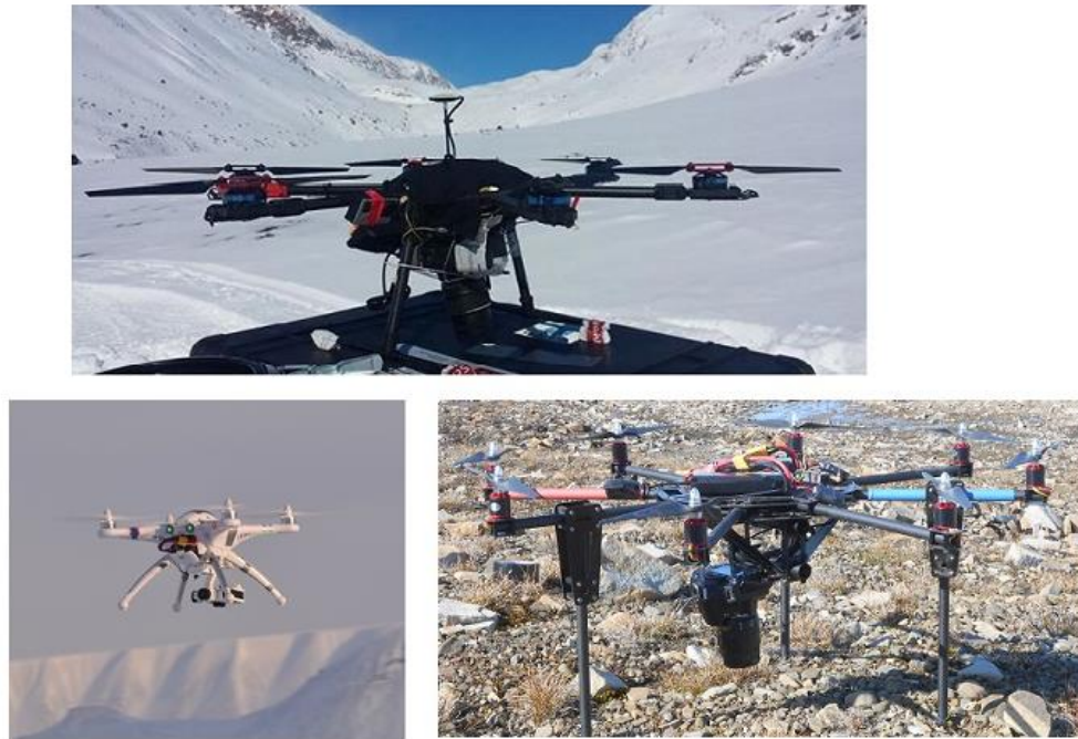
Figure 8: Pictures of the used multi-rotors UAVs. The Walkera X350 Pro (bottom-left), the DJI s900 Spreading Wings (top-center) and the custom build octocopter (bottom-right).
